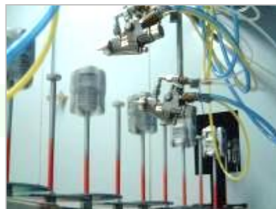
Medium workpiece conveyor type for painting car bumpers, doors, lights, TV frames, etc.
