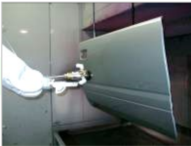
Small workpiece spindle-type for painting car bodies, etc.
