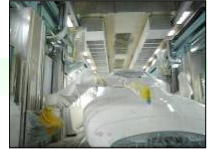
Large workpiece type for painting rail cars, bogies, building components, etc.
